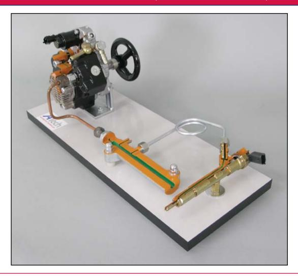
This model shows an accurate cross-section of the high pressure (1300 bar) fuel system known as common rail. This circuit consists of a radial piston pressure pump, one delivery manifold, and an electro injector, all connected via high pressure hoses.
