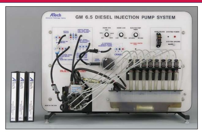
This GM 6.5L Diesel Injection Pump System (model 6601) trainer presents the "real-world" operation and study of the Stanadyne rotary diesel fuel injection pump. The program provides an operational study of the diesel fuel injection system. The program includes courseware for use by students and instuctors.
